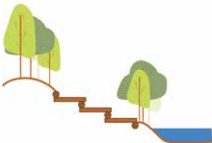
Crib logs to prevent erosional runoff
