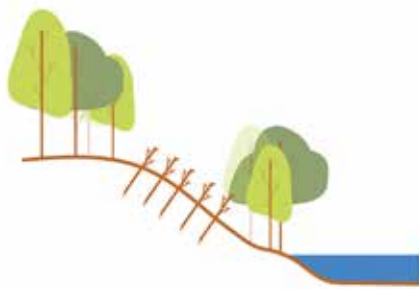
Live staking for root stabilization on slopes
